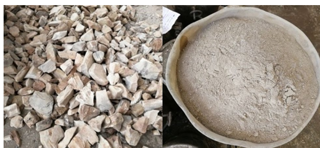
Fig. 3 The OSA obtained after crushing, burning, and grinding
