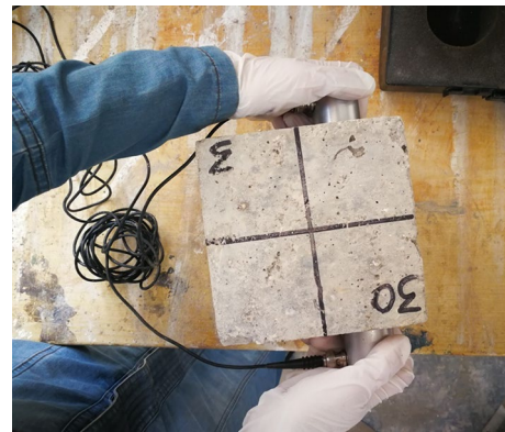
Fig. 7 UPV direct test
