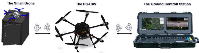
Figure 8. The PC-UAV relay station system
