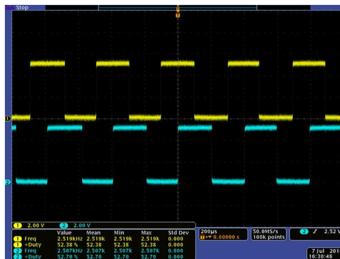
Fig. III.10: Encoder A and B Outputs at the Rated Voltage of the Preferred DC Motors (Pololu Corporation, 2022b)
