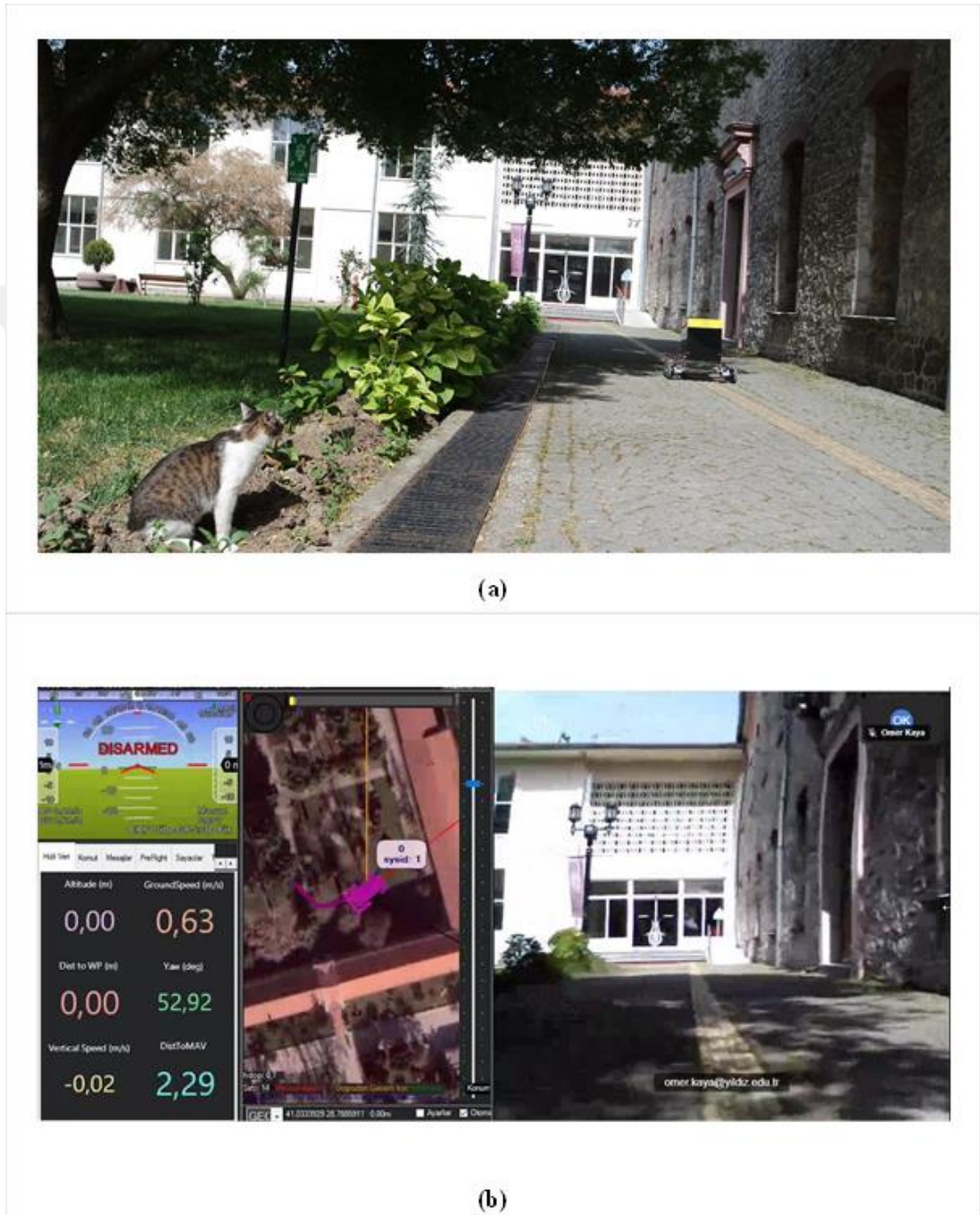
Fig. IV.6: A Sample Scenario, a) The robot is on duty outside, b) The remote operator monitors on the remote-control station screen what the robot sees and steers the robot remotely.
