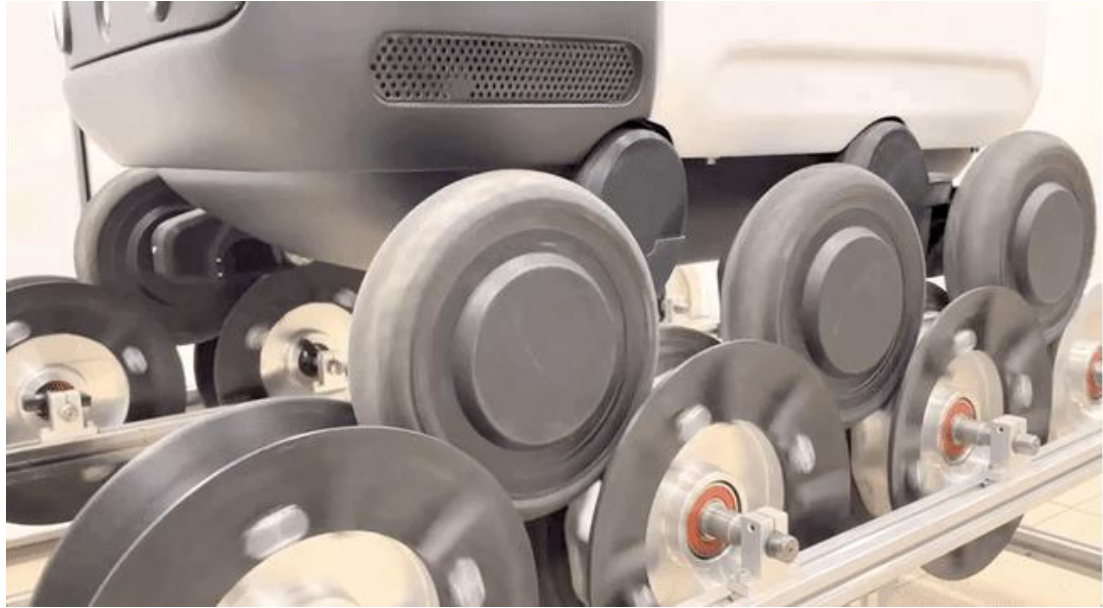
Fig. II.20: Suspension Test Device (Yandex Self-Driving Team, 2021)
