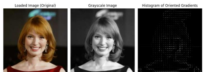
Fig. 3. Example of feature extraction step by step of HOG descriptor.
