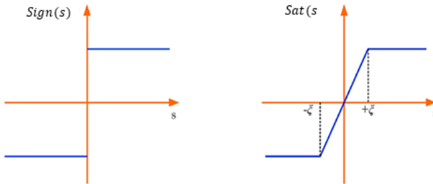
Figure 2: Linear saturation function approximation of the sign function.
