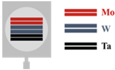
Fig. 2. Schematic illustration of the holder developed
