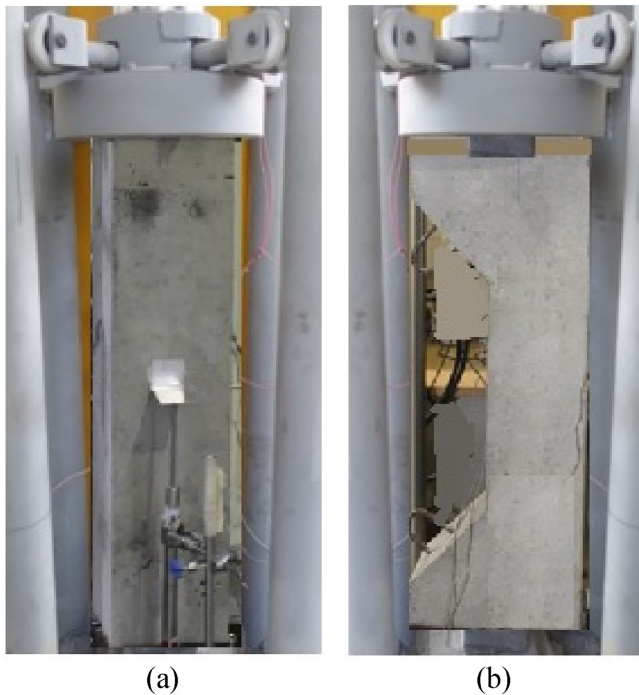
FIGURE 4 Actual photo of the columns' arrangement and test setup under. (a) Concentric load. (b) Eccentric load.
