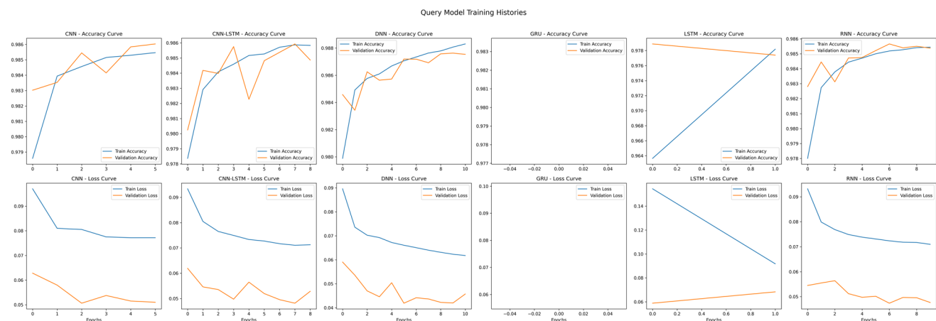
Fig. 13 Model training results on FWF dataset: Accuracy evolution (upper panel) and loss reduction (lower panel) during training/validation for compared architectures. Yellow lines indicate validation set performance
