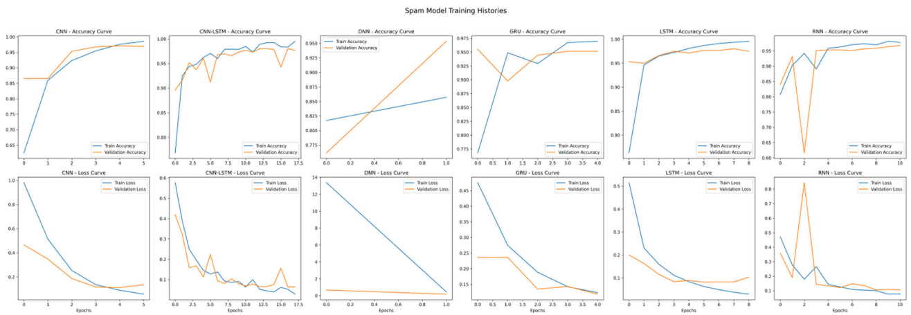
Fig. 16 Model training results on SMSSpamCollection dataset: Accuracy evolution (upper panel) and loss reduction (lower panel) during training/validation for compared architectures. Yellow lines indicate validation set performance
