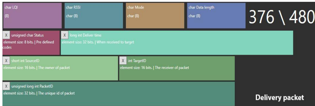
Figure 4.9: An example for data header structure
