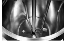
Fig. 10.2 Batch pan fryer with a central stirring blade. Courtesy of GEA Group, Düsseldorf, Germany.
